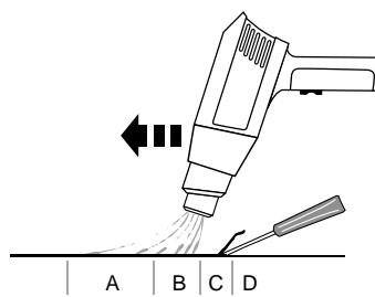
**Note:** Do not use the heat gun on surfaces that can be damaged by heat, such as vinyl-coated paneling, siding or window frames.
