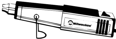
**NOTE:** Keep the nozzle pointed up after shutdown, either for a short break or for storage. If the nozzle is pointed down, the residual heat rises into the motor space and shortens the life of the unit. Avoid laying the unit on the side after shutdown. The heat will remain in the unit and cooling will take longer. Store the unit only after the nozzle is cool to touch. Unplug the unit before storing to prevent accidental start up.
